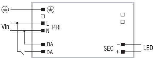
PUSH SWITCH diagram - Collegamento PUSH SWITCH
